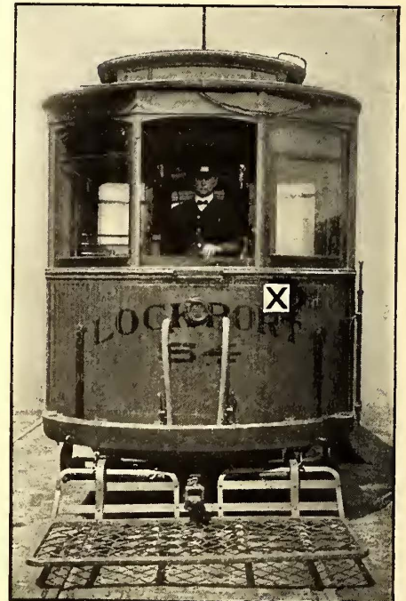
PLATE 21.—FRONT END EXTRA TRAIN, CARRYING WHITE SIGN WITH BLACK X, BY DAY—SEE RULE I-13
