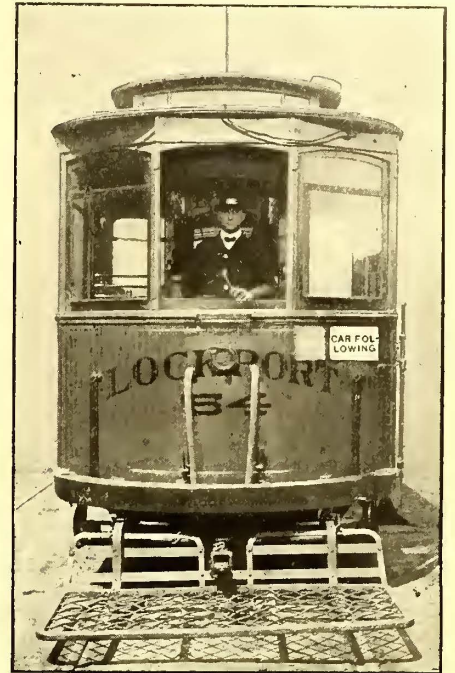
PLATE 17.—FRONT END REGULAR TRAIN, CARRYING SECOND SECTION SIGNALS, GREEN AND RED DASH SIGN, BY DAY—SEE RULE I-12
