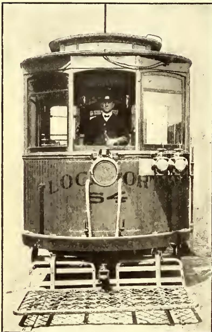
PLATE 19.—FRONT END REGULAR TRAIN, CARRYING SECOND SECTION SIGNALS, GREEN LANTERN, RED DASH SIGN AND LANTERN, BY NIGHT—SEE RULE I-12
