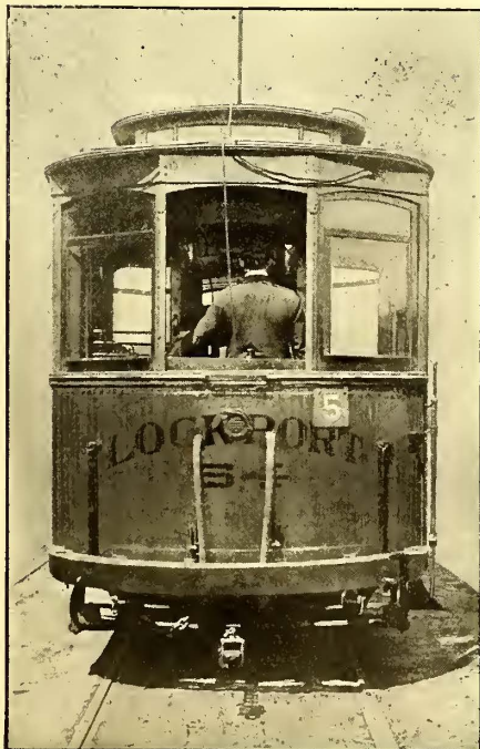
PLATE 14.—REAR END REGULAR TRAIN, WITH RED DASH SIGN, BY DAY—SEE RULE I-11
