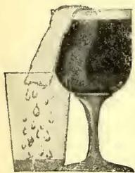
PRINCIPLE OF OPERATION OF THE CAPILAR OIL FILTER
