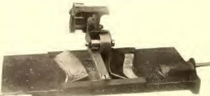
FIG. 3.—OPERATING WHEEL THROWING SWITCH
