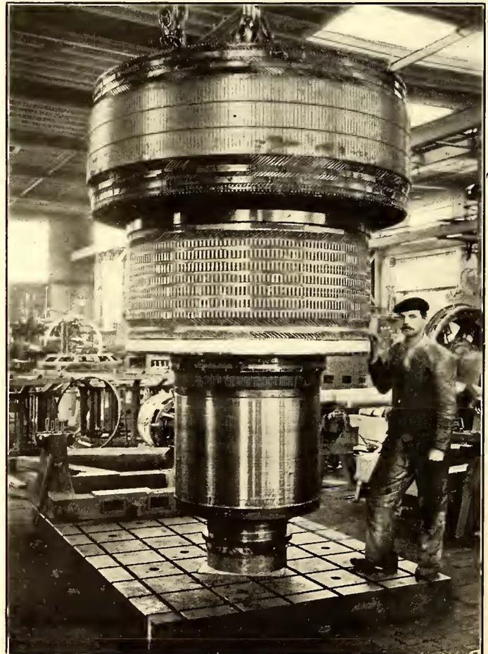
FIG. 3.—VERTICAL MOTOR GENERATOR SET, WITHOUT FRAME
