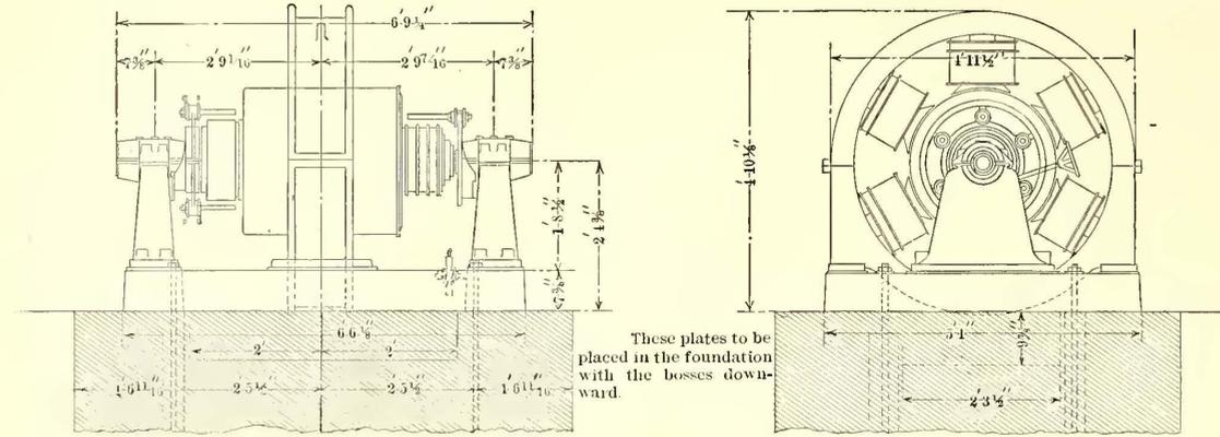
FIG. 7.—ROTARY CONVERTER
