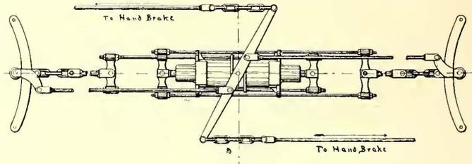
FIG. 3.—DUPLIX JAM CYLINDER, SHOWING HAND BRAKE CONNECTIONS
