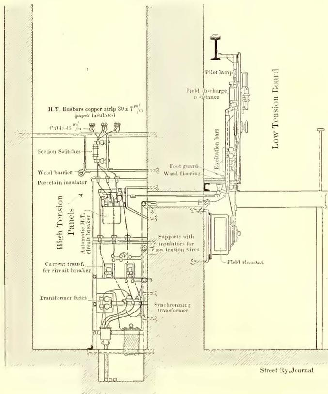
FIG. 14.—SECTION THROUGH ALTERNATOR PANEL AT LAXEY
