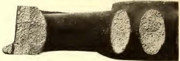
FIG. 1.—FUSED WHEEL BROKEN TO SHOW APPEARANCE OF FRACTURES IN TIRE AND SPOKES
