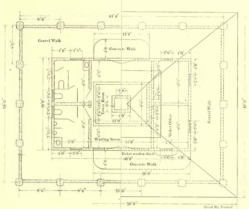
FIG. 2.—PLAN OF COMBINATION WAITING AND SUB-STATION BUILDING
