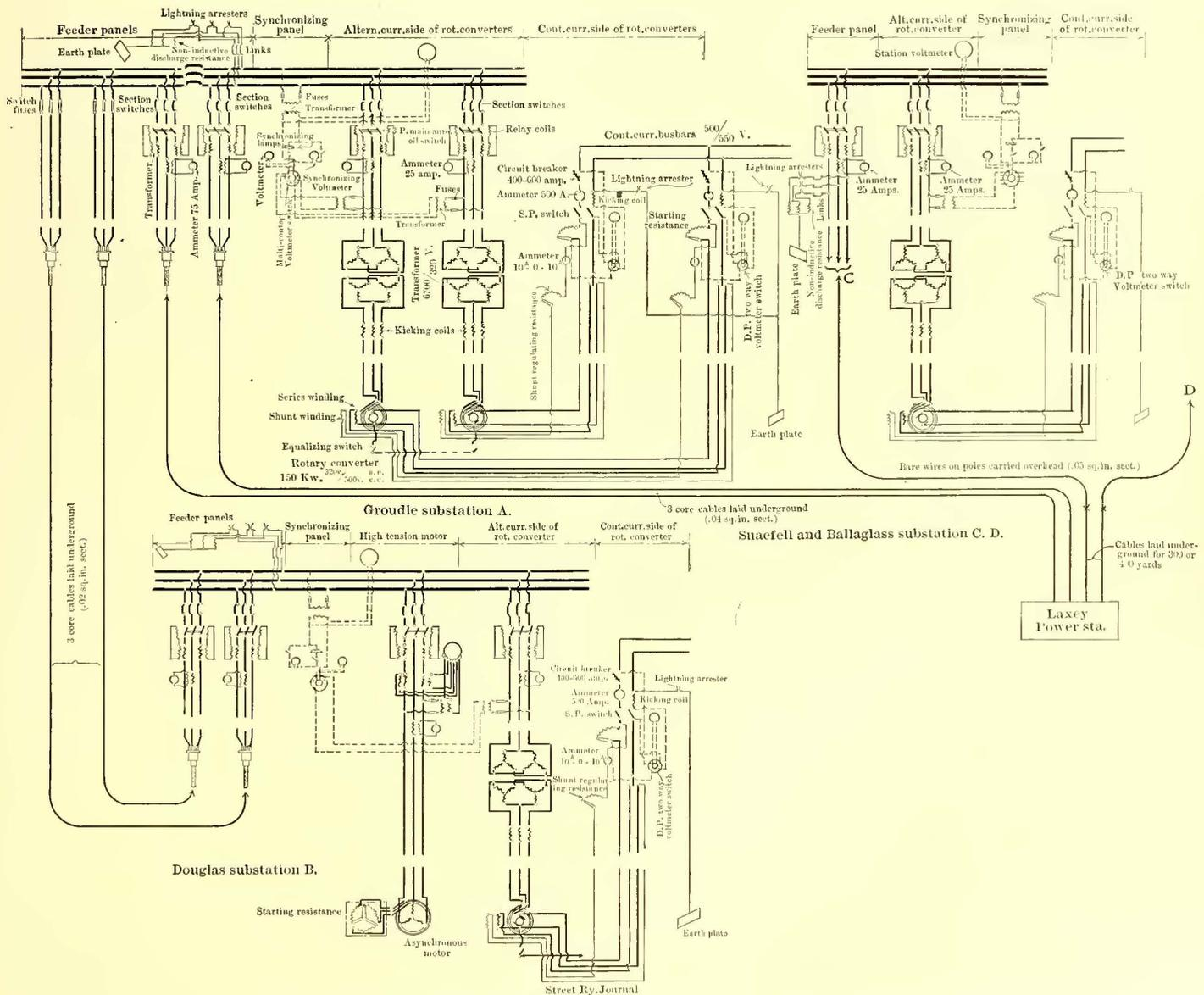
FIG. 13.—DIAGRAM OF SWITCHBOARD CONNECTIONS AT BALLAGLASS SUB-STATION
