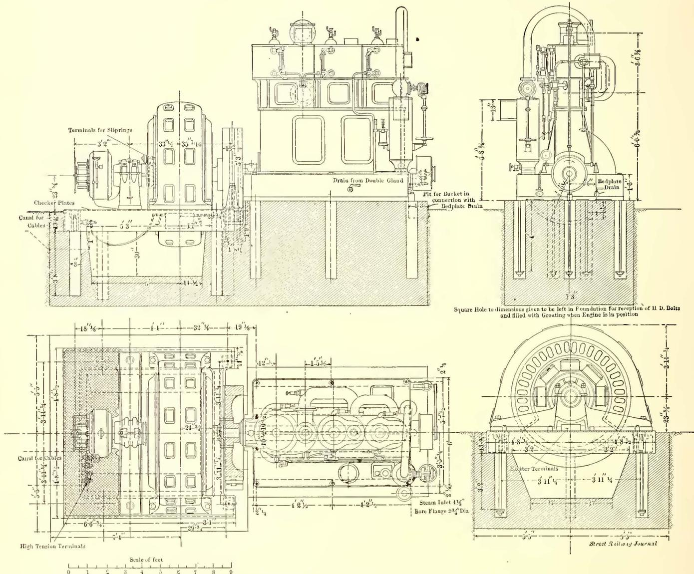
FIGS. 3 AND 4.—300-KW HIGH-TENSION GENERATOR SET AT LAXEY
