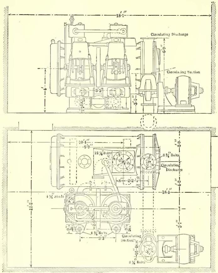
FIG. 18.—PLAN AND END ELEVATION OF CONDENSER PUMPS
