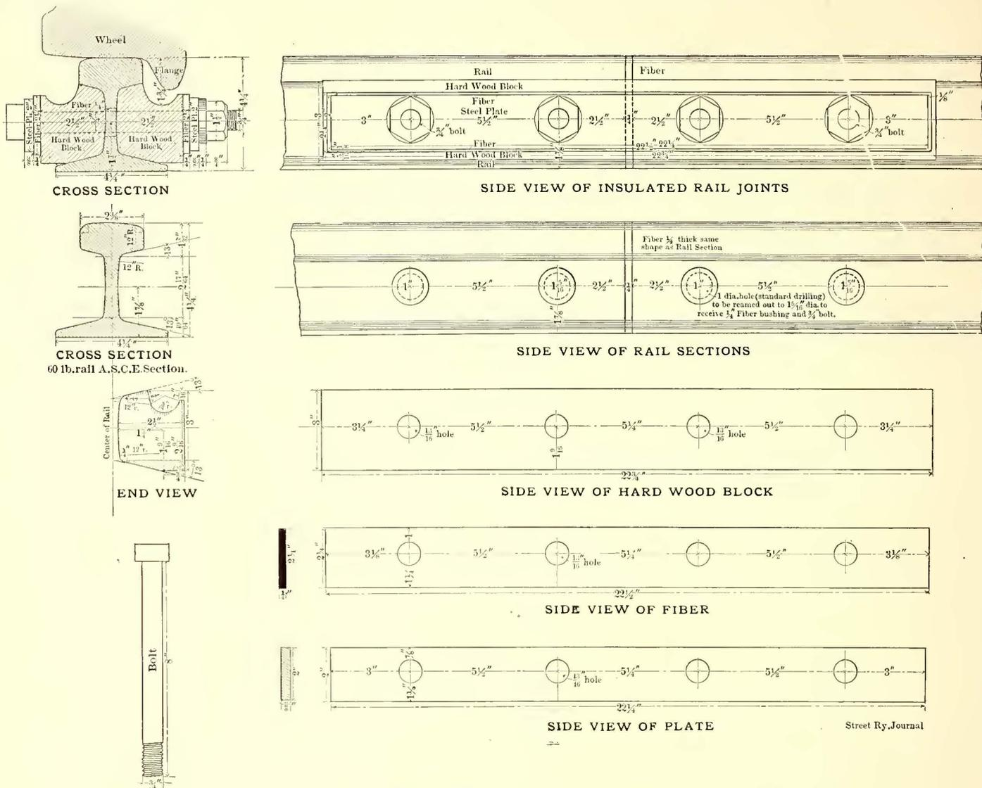
FIG. 3.—INSULATING RAIL JOINTS USED IN CONNECTION WITH THE ALTERNATING-CURRENT BLOCK SIGNAL SYSTEM
