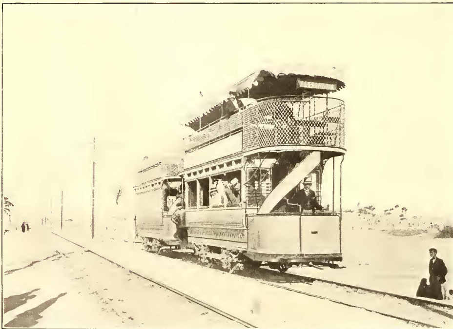
VIEW OF THE MAIN LINE AND TYPE OF DOUBLE-DECK CARS USED, SHOWING FIRST-CLASS MOTOR CAR AND SECOND-CLASS TRAILER
