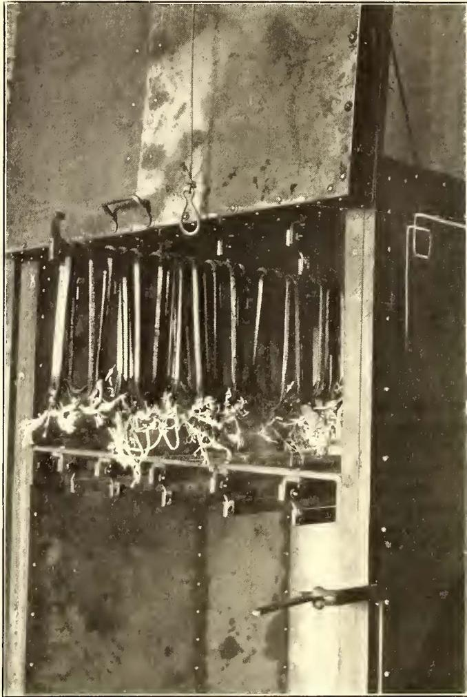
FIG. 13.—BAKING OVEN, WITH RACK PARTLY PULLED OUT
