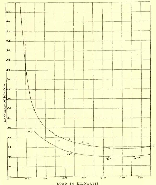
FIG. 3.—500-KW CURTIS TURBINE AT NEWPORT, R. I., CURVES SHOWING STEAM CONSUMPTION (WATER RATE PER KW-HOUR) AT DIFFERENT LOADS, WITH AND WITHOUT SUPERHEAT—INITIAL PRESSURE 145-LB. GAGE
