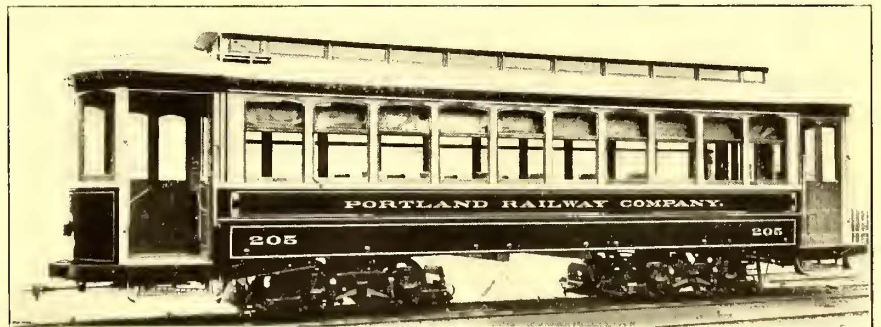
SEMI-CONVERTIBLE CAR USED BY PORTLAND RAILWAY COMPANY.
