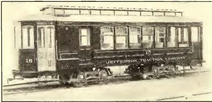
COMBINED SEMI-CONVERTIBLE AND BAGGAGE CAR FOR THE JEFFERSON TRACTION COMPANY
