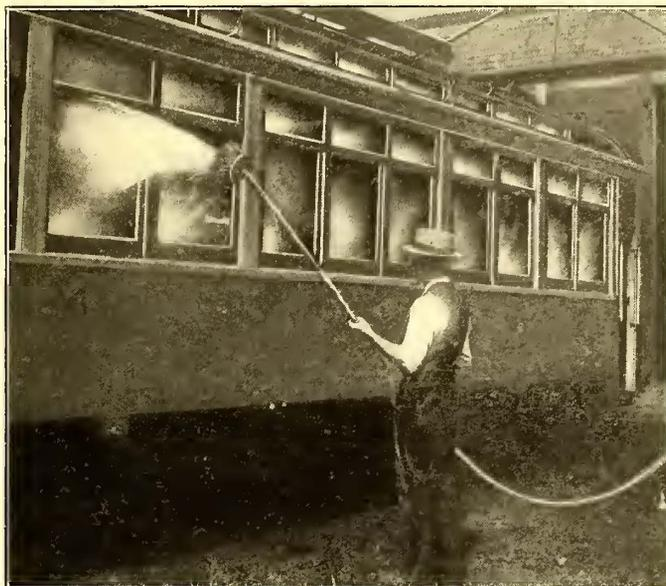
METAL CAR BRUSH, WITH ATTACHMENT FOR SPRAYING
