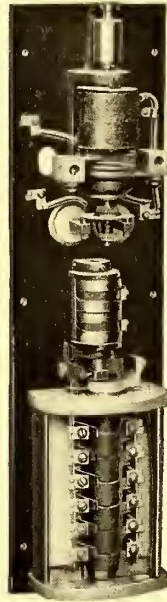
FIG. 7.—TRIP MAGNETS ON TOP OF CUT-OUT SWITCHES
