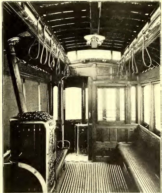
INTERIOR OF THE VINCENNES CAR, SHOWING ACCELERATOR DOOR, VESTIBULE, SEATING ARRANGEMENT AND HEATER
