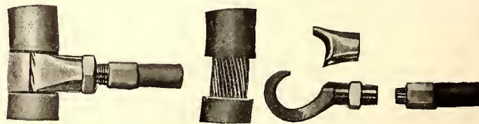
FIGS. 1 AND 2.—ASSEMBLY AND PARTS OF TAP JOINT
