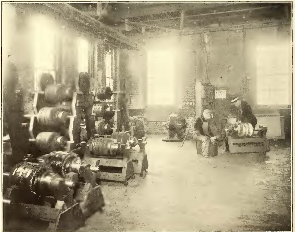
VIEW IN TESTING CORNER OF THE ELECTRICAL REPAIR DEPARTMENT, SHOWING ALSO SCHEME OF ARMATURE STORAGE IN USE
