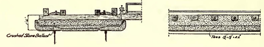
Ballasted Floor Type E (Concrete Steel) Weight Inner Stringer 1300 o per lin foot Outer 1200 Total 2500
