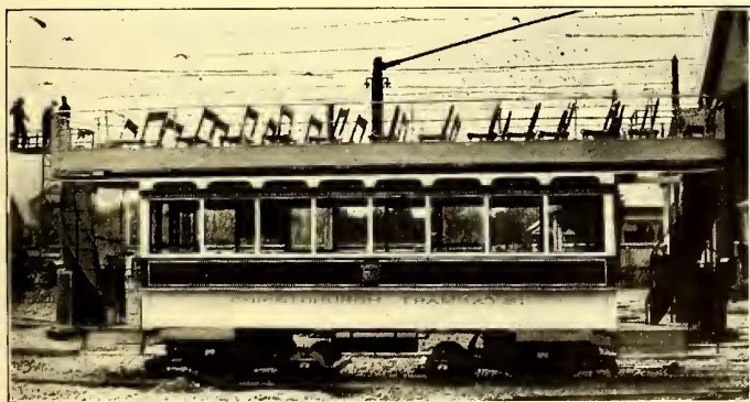
TYPES OF THE DOUBLE-DECK CAR AND DOUBLE-VESTIBULE CLOSED CAR USED ON THE CHRISTCHURCH TRAMWAYS
