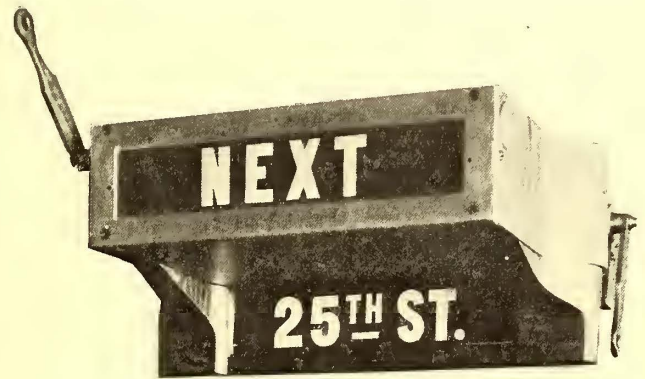
VIEW OF STATION INDICATOR IN SERVICE
