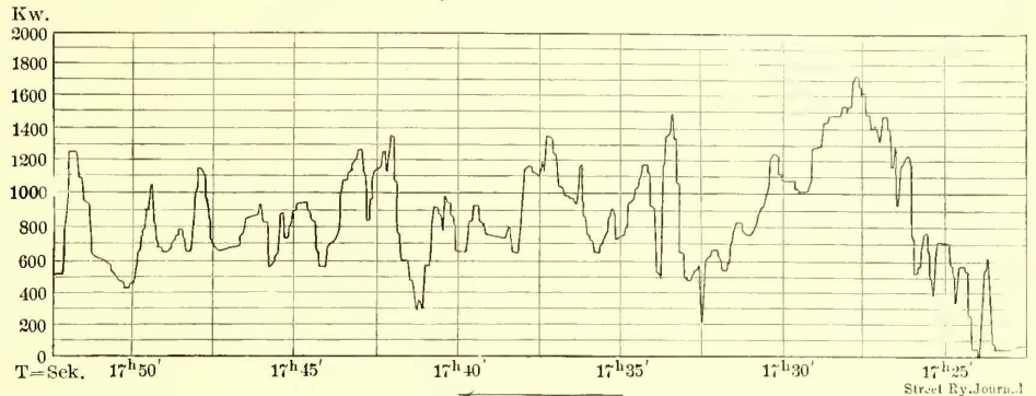
FIG. 3.—LOAD DIAGRAM, TAKEN AT THE MORBEGNO POWER STATION
