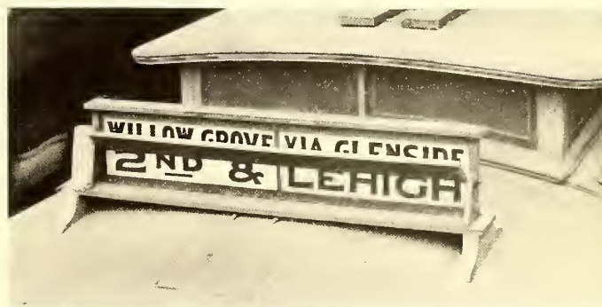
HOOD DESTINATION SIGN, SHOWING METHOD OF CHANGING DESIGNATION BY MEANS OF MOVABLE FLAP
