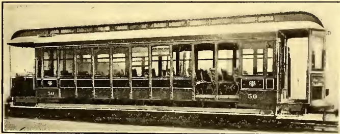
CONVERTIBLE CAR FOR THE SHREVEPORT TRACTION COMPANY, SHOWING TWO OF THE PANELS REMOVED
