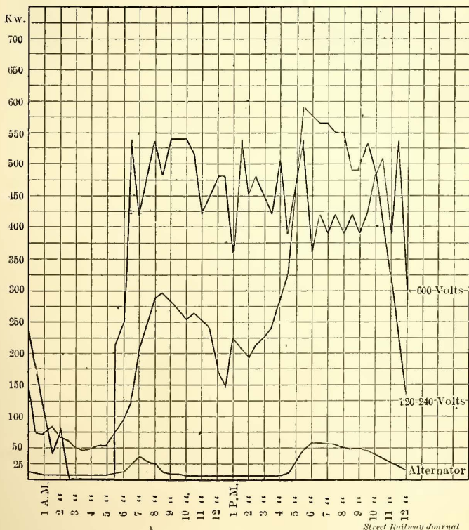
LOAD CURVE OF EDISON ELECTRIC ILLUMINATING COMPANY, TOPEKA, KAN., WITHOUT BATTERY ON RAILWAY LOAD
