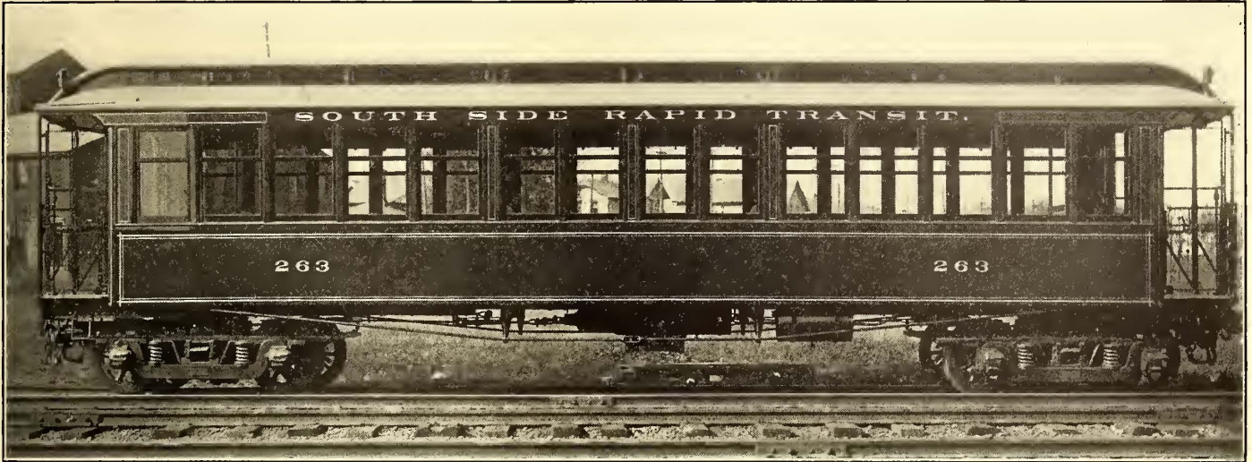
FIG. 1.—AN EXAMPLE OF THE LATEST TYPE OF CAR FOR THE SOUTH SIDE ELEVATED RAILROAD COMPANY, OF CHICAGO, EMBRACING NEW STYLE OF MOTORMAN'S CAB AND DOUBLE FOLDING GATE
