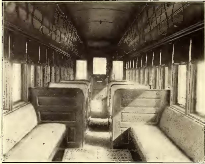
FIG. 4.—VIEW OF CAR INTERIOR, SHOWING THE LONGITUDINAL SEATING AND CROSS SEATS IN CENTER
