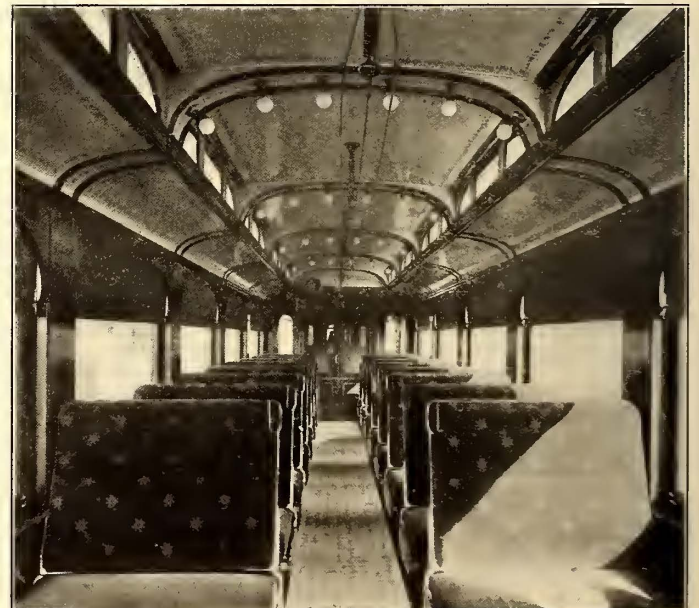
INTERIOR VIEWS OF THE OPEN AND CLOSED CARS OF THE WESTERN MASSACHUSETTS STREET RAILWAY COMPANY, SHOWING THE SEATING ARRANGEMENT AND THE UNUSUAL METHOD OF CAR LIGHTING
