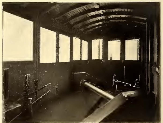
INTERIOR OF SNOW SWEEPER, SHOWING THE CONVENIENT ARRANGEMENT OF THE LEVERS FOR RAISING AND LOWERING THE BROOMS AND BRUSH-BOARDS
