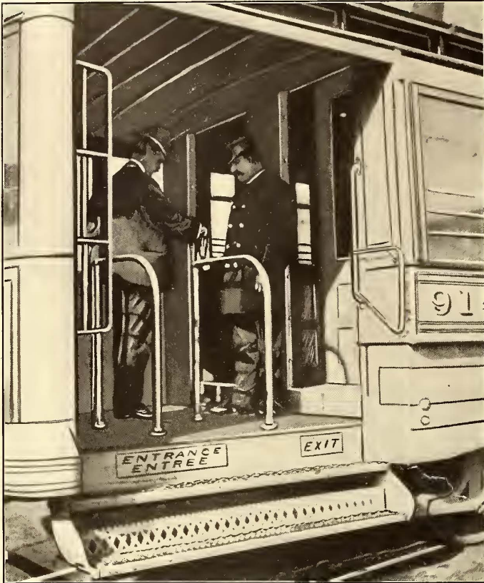
REAR PLATFORM OF "PAY-AS-YOU-ENTER" CAR, SHOWING POSITION OF CONDUCTOR AND PASSENGER WHEN PAYING FARE
