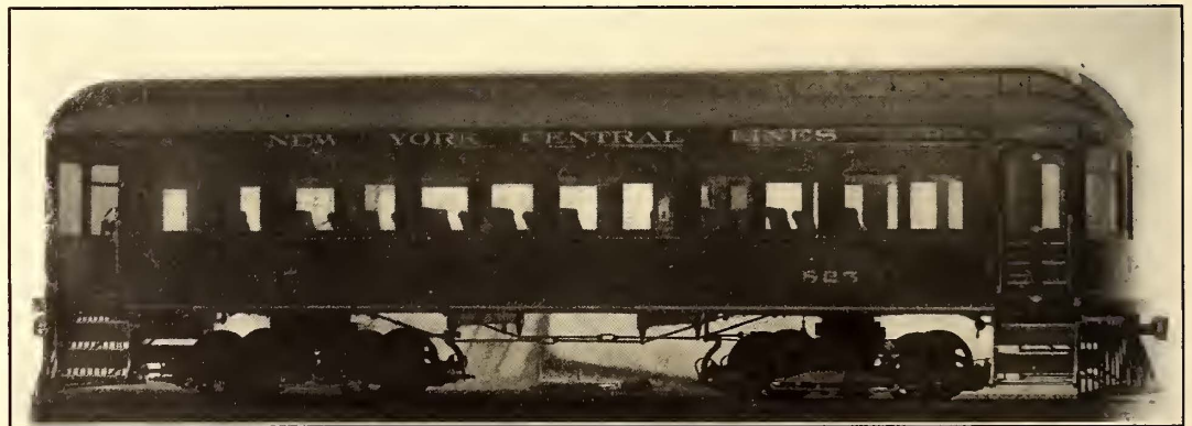
GASOLINE-ELECTRIC CAR, BUILT FOR OPERATION ON THE LAKE SHORE & MICHIGAN SOUTHERN RAILWAY
