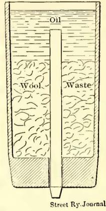
FIG. 2.—GREASE BOX WITH OIL CUP INSIDE; ALSO SECTION OF OIL CUP
