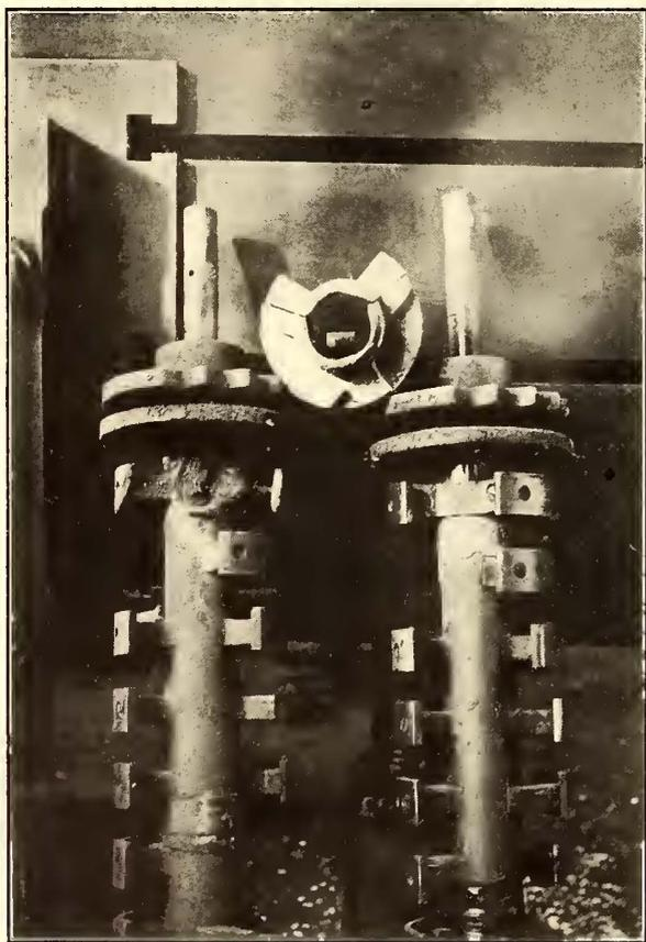
FIG. 4.—A BURNED CONTROLLER AND A REPAIRED ONE, WITH REPAIR CASTING
