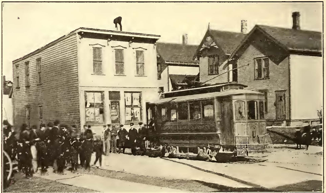
ONE OF THE ASHTABULA RAPID TRANSIT COMPANY'S CARS MOVING A HOUSE AT ASHTABULA, OHIO
