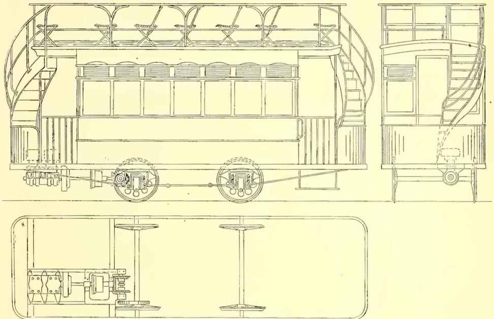
ELEVATIONS AND PLAN OF GASOLINE STREET CAR
