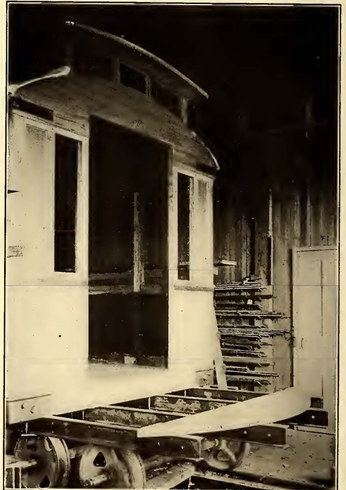
FIG. 9.—END OF CAR, SHOWING I-BEAMS, UPON WHICH THE PLATFORM AND VESTIBULE ARE BUILT
