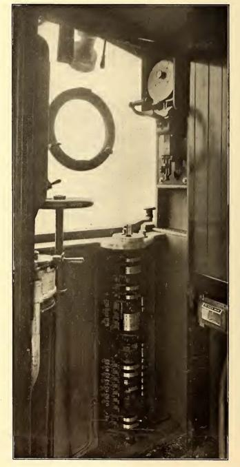
FIG. 3.—VIEW OF CONTROLLING APPARATUS ON MULTIPLE-UNIT TRAIN
