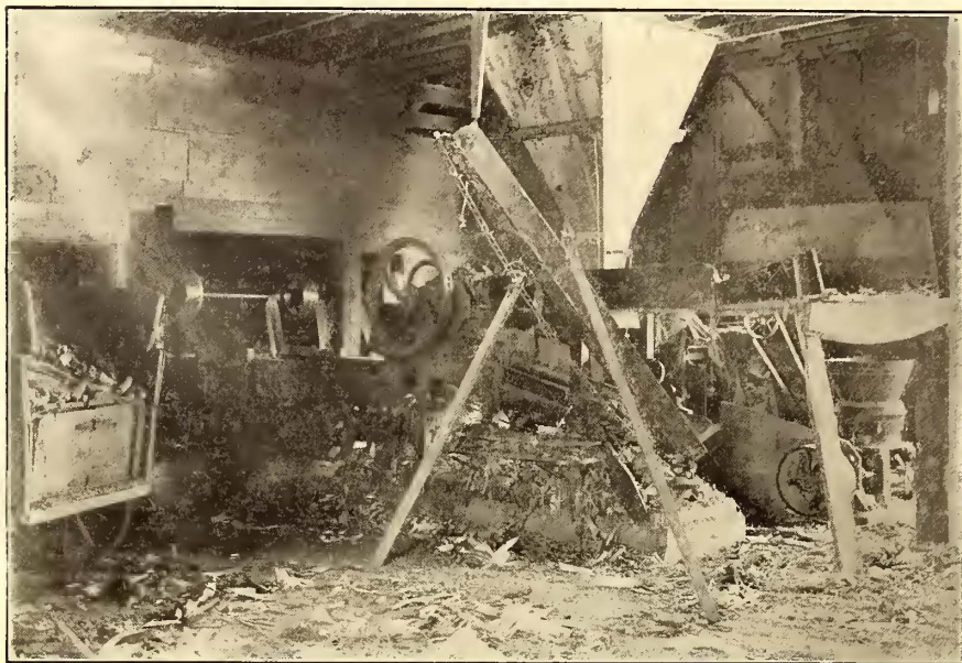
A CORN SHREDDER AND CRUSHER DRIVEN BY A 15-HP MOTOR
