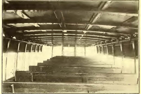
VIEW FROM THE REAR OF THE UPPER DECK, SHOWING SIDE CURTAINS AND FRONT SASH
