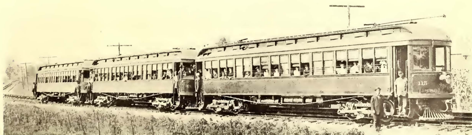
THREE-CAR TRAIN USED FOR HANDLING HEAVY TRAFFIC, SCIOTO VALLEY. THIS TRAIN HAS SEATING CAPACITY OF 210 PASSENGERS
