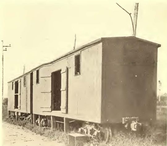
PORTABLE SUB-STATION, COLUMBUS, DELAWARE & MARION
