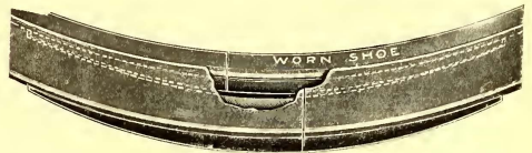
FIG. 4.—WORN SHOE IN NEW SHOE, SHOWING LAP JOINT
