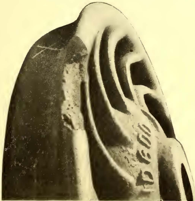
WHEEL WITH BROKEN FLANGE
