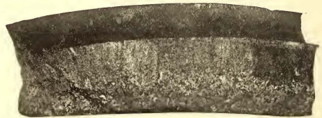
SECTION OF WHEEL, SHOWING INCIPIENT FRACTURE
