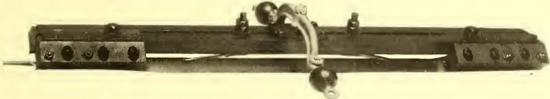
FIG. 3.—TROLLEY SWITCH FOR SIGNAL SYSTEM
