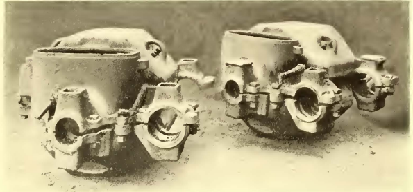
FIG. 1.—STEEL MOTOR FRAME WELDED
