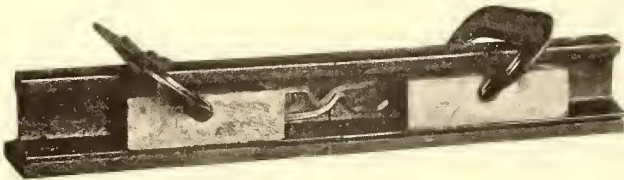
APPLICATION OF COPPER BEFORE WELDING
