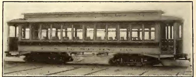
SEMI-CONVERTIBLE CAR FOR FITCHBURG & LEOMINSTER STREET RAILWAY
