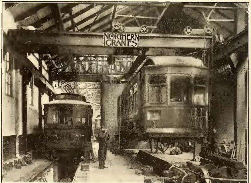
TWO TROLLEYS FOR LIFTING CAR BODY
