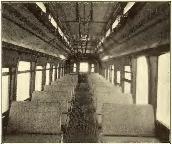
INTERIOR OF SEMI-CONVERTIBLE CAR FOR WEST CHESTER
