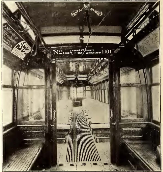
INTERIOR OF SEMI-STEEL CAR, SEEN FROM SMOKING COMPARTMENT
