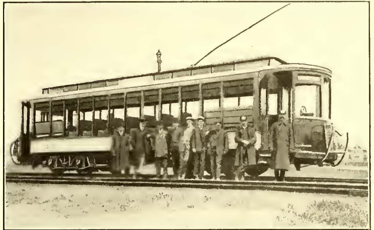
FIG. 6.—TYPE OF FOUR-MOTOR CAR TESTED
