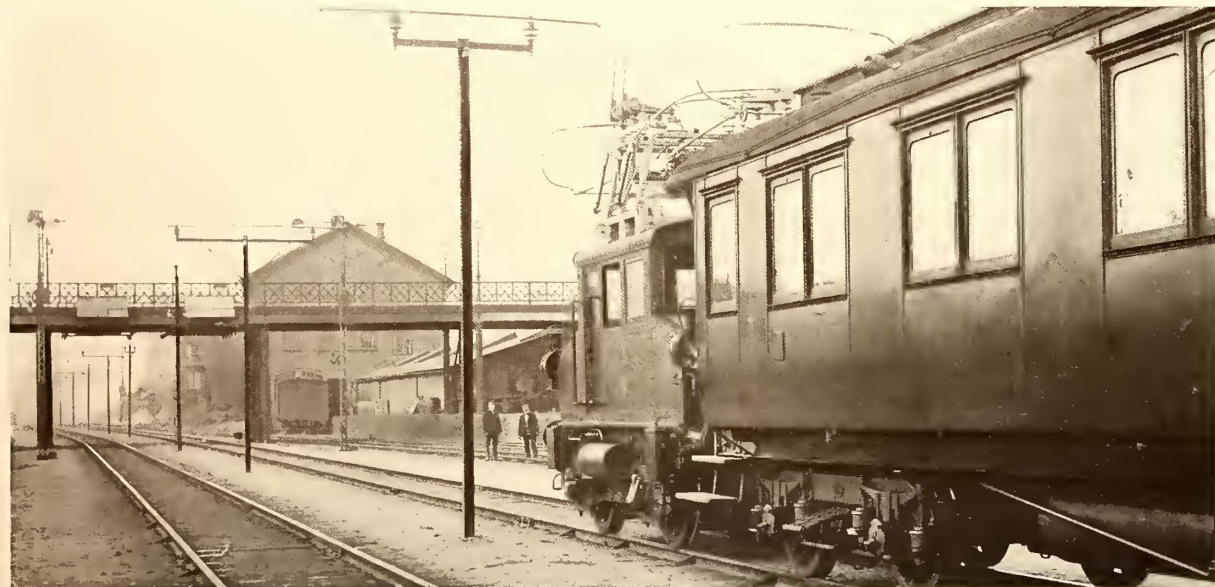
WESTINGHOUSE ELECTRIC LOCOMOTIVE WITH OERLIKON OVERHEAD COLLECTOR HAULING TRAIN ON GOVERNMENT RAILWAYS AT STOCKHOLM
