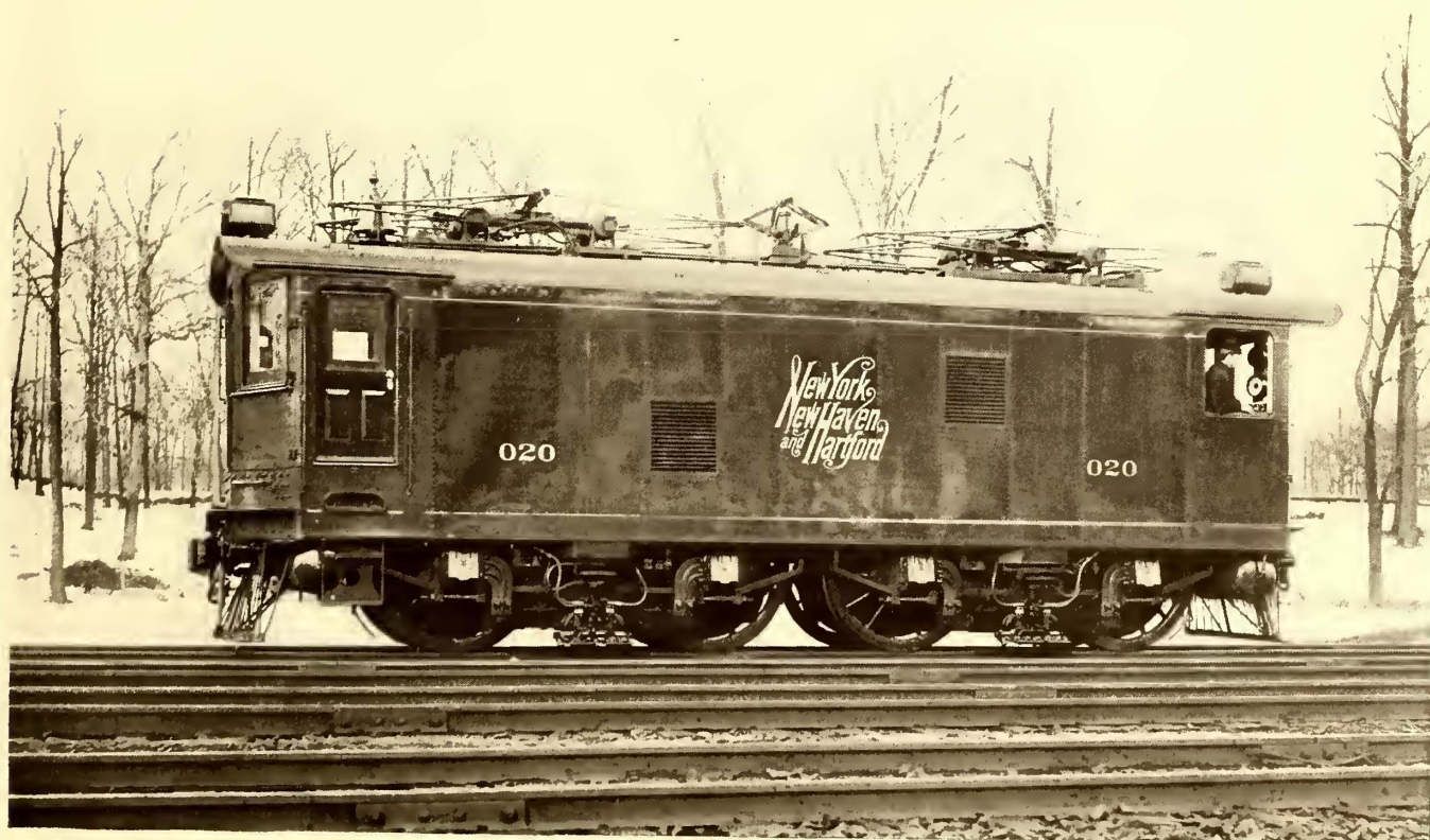
LOCOMOTIVE WITH SINGLE-PHASE PANTOGRAPH TROLLEY LOWERED, NEW HAVEN RAILROAD
