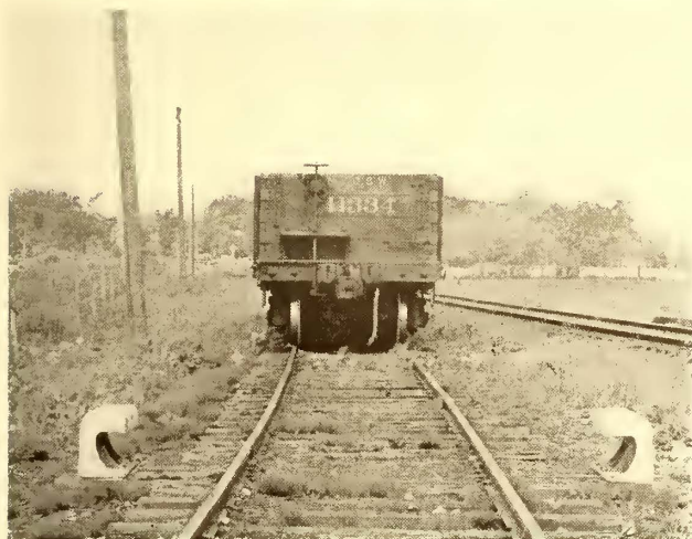
TELL-TALE USED FOR GAGING TRAINS BEFORE PASSING ON TO THIRD-RAIL SECTIONS, WEST SHORE RAILROAD
