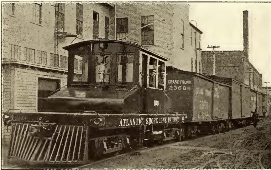
ELECTRIC LOCOMOTIVE HAULING A TRAIN OF STANDARD FREIGHT CARS OVER A MILL SIDING
