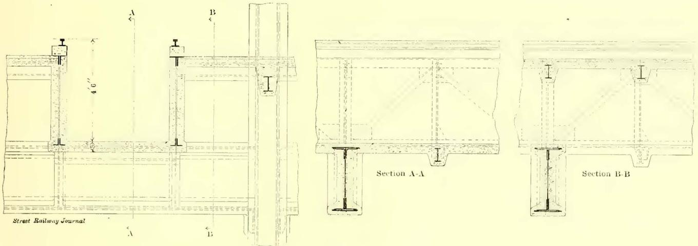
SECTION AND ELEVATION OF PITS
