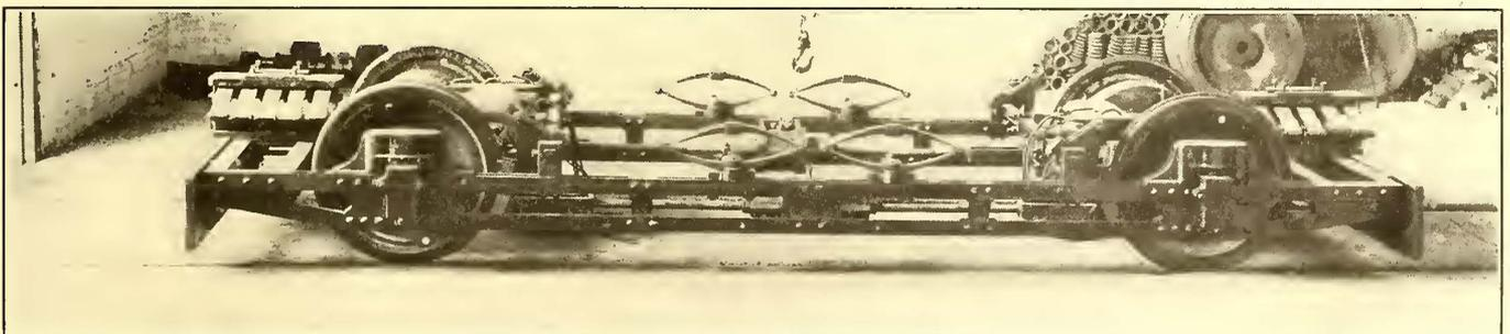
SIDE VIEW OF TRUCK, SHOWING NOVEL ARRANGEMENT OF SPRINGS
