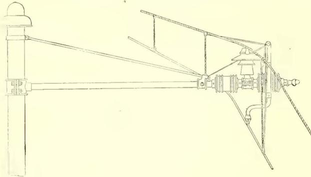
FIG. 1.—BRACKET CONSTRUCTION FOR CURVES
