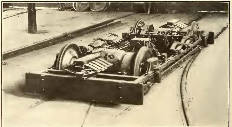
END VIEW OF TRUCK, SHOWING METHOD OF MOUNTING MOTORS AND AIR COMPRESSOR ON TRUCK; ALSO ARRANGEMENT OF SPRINGS
