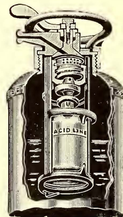
SECTIONAL VIEW OF UPPER PART OF EXTINGUISHER
