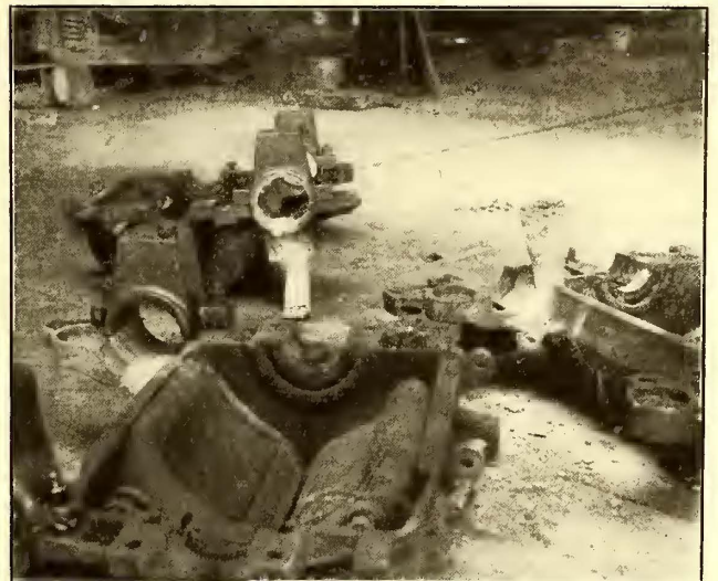
MOTOR CASES WELDED BY THERMIT
