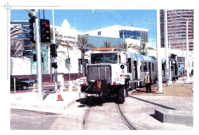
The first Light Rail Vehicle clearance test began on January 27, 2009 during which a new 2550 Ansaldobreda Vehicle was being pulled along the entire alignment to ensure that the vehicle clears all of the stations and other physical elements.
