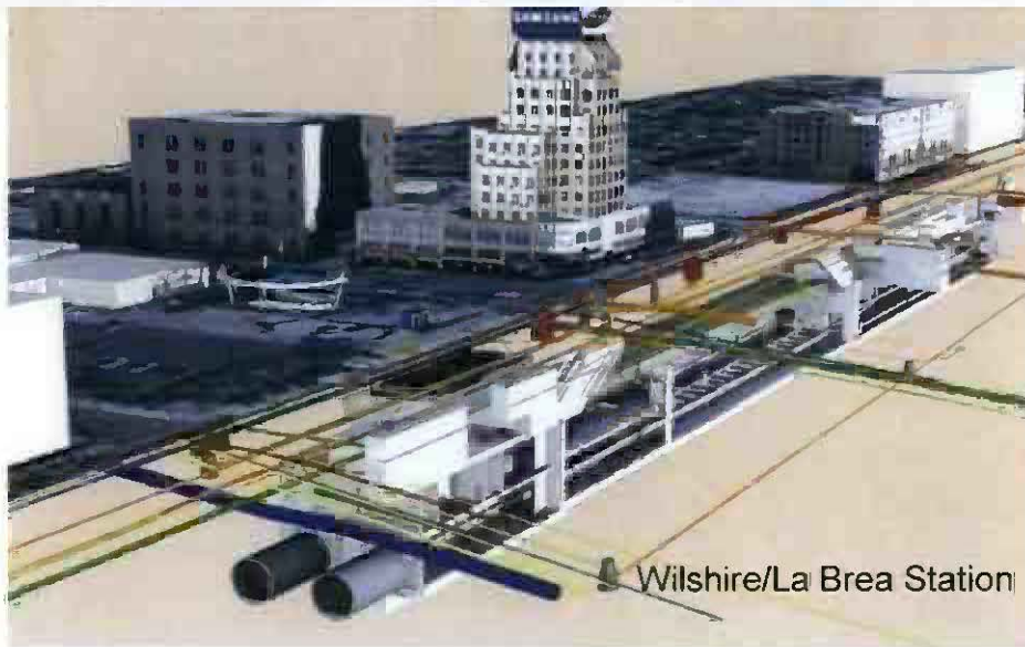
Relocated Utilities (Clear of Shoring Piles)
