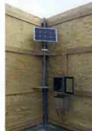
Placement of Geotechnical Instrumentation before Shaft Construction
