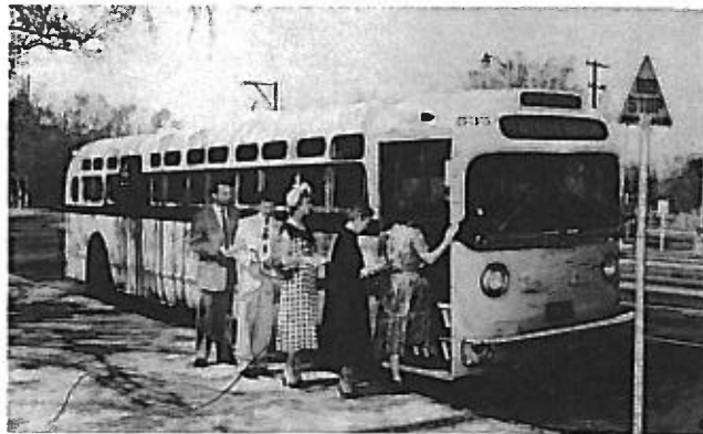
MODERN CURB-LOADING BUSES offer passengers greater convenience and safety. Traffic hazards are eliminated when coaches load and discharge riders directly at designated stops next to curbs.
