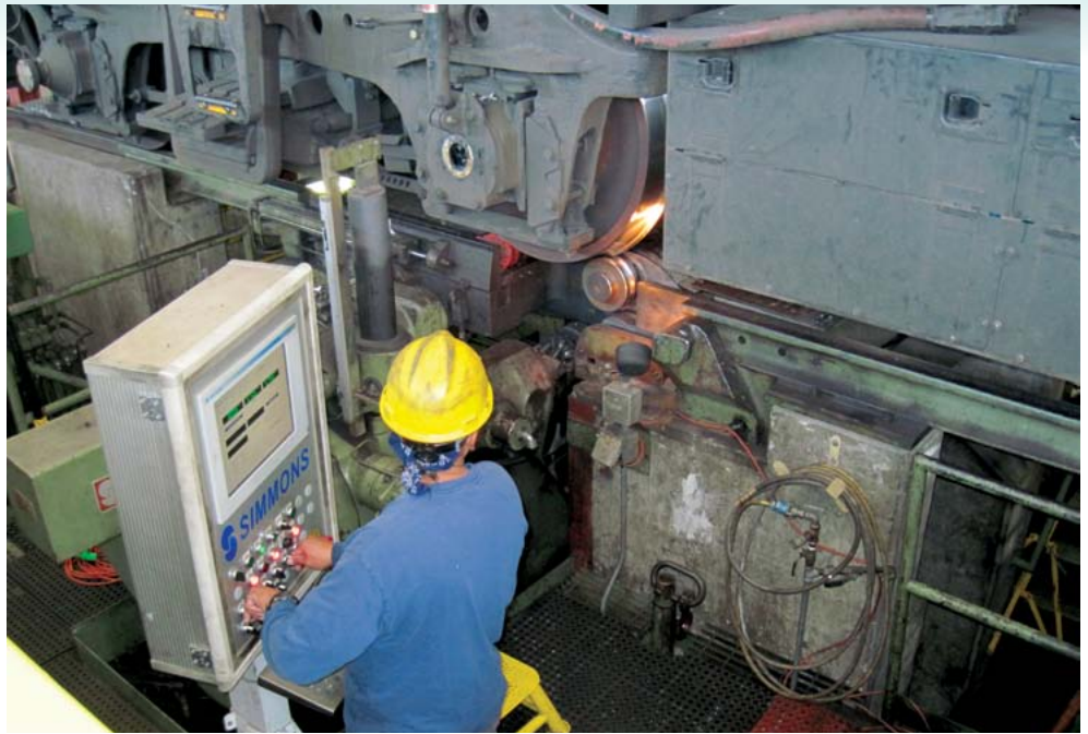
A mechanic operates a wheel-truing machine at Metrolink's Central Maintenance Facility in Los Angeles.
